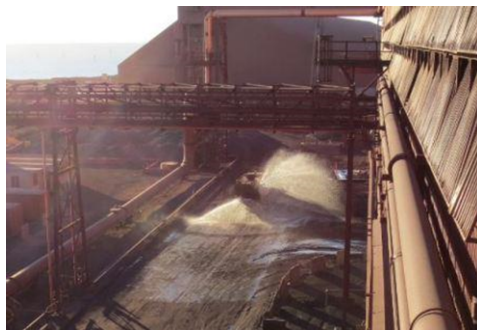
Use of dust suppressant chemicals & water sprays at transfer points
