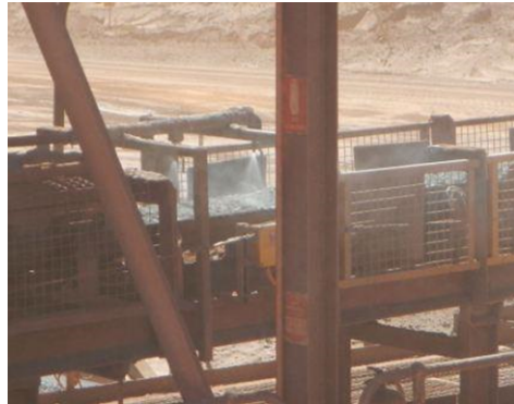
Use of dust suppressant chemicals & water sprays at transfer points
