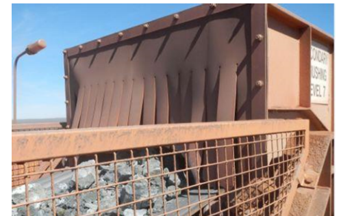
Enclosure of dusty machines & transfer points
