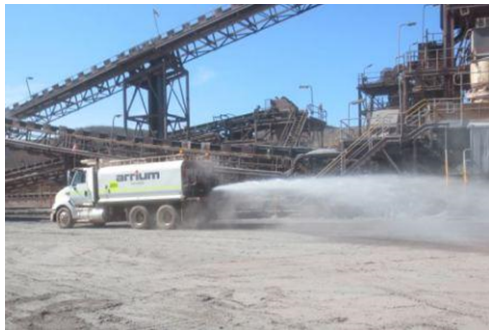
Use of dust suppressant chemicals & water sprays at transfer points
