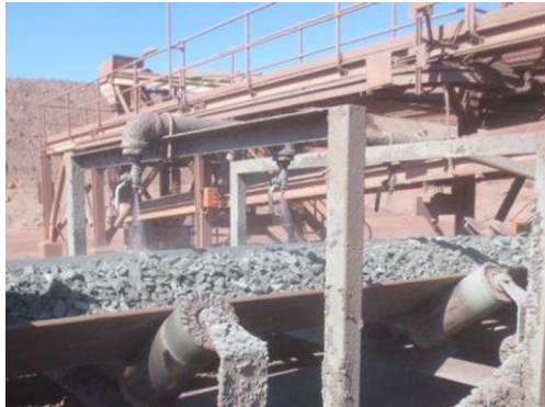
Use of dust suppressant chemicals & water sprays at transfer points
